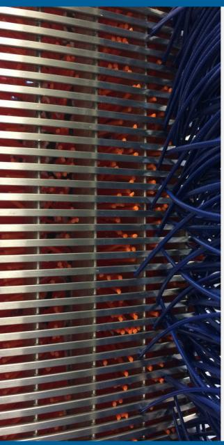
The screen unit consists of cylindricalshaped wedgewire screen, an external and internal brush cleaning system, flow baffle, and brush drive assembly with controls. Gravity, siphon, or pumping is used to convey water through the screen.
